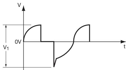
Choice of voltage:  $V_1 \leq V_{\text{peak}}$
